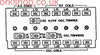
NOTE:-MW. S.W. AND 31 M. AE. TRIMMERS UNDER CHASSIS (31 M. TRIMMER ADJACENT TO L6) LFT. PRIMARIES UNDER CHASSIS. LFT. SECONDARIES ABOVE CHASSIS.
