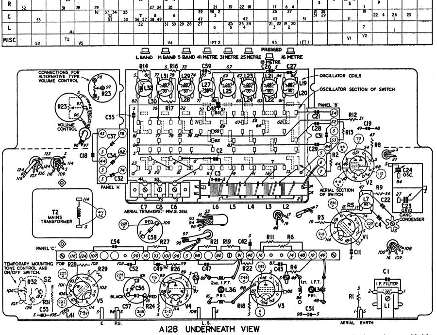
Voltages shown on these layout diagrams were measured between the test points and chassis (except where shown otherwise) using an Avometer Model 7. The receiver was switched to M.W. and working on 245 volts mains supply, connected to the 240-260 volt tap, under no signal conditions. Variations may however occur without affecting the performance of the receiver.
