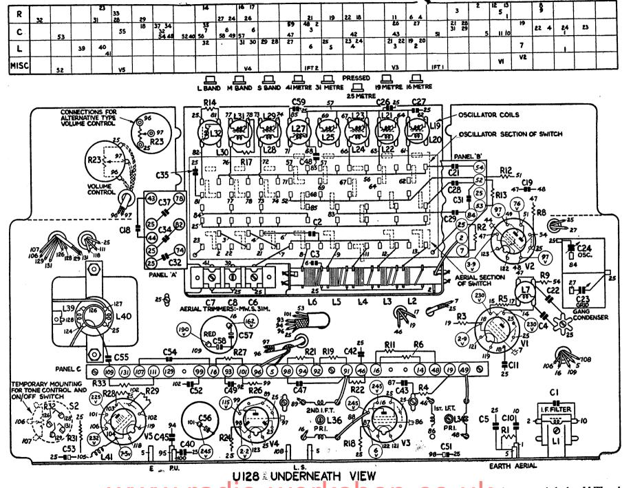
Voltages shown on these diagrams were measured between test points and chassis, using an Avometer, Model 7. The receiver was switched to M.W. and was working on 245 volt A.C. mains supply, connected to the 250 volt tap, under no signal conditions. Variations may however occur without affecting the performance of the receiver.
